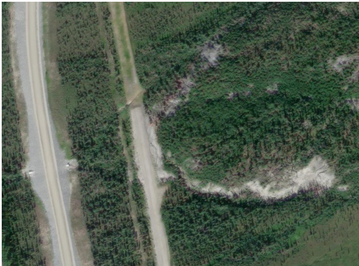
Figure 4.1.4-14: FDL-A Nearing/Touching the Abandoned Section of the Dalton Highway
