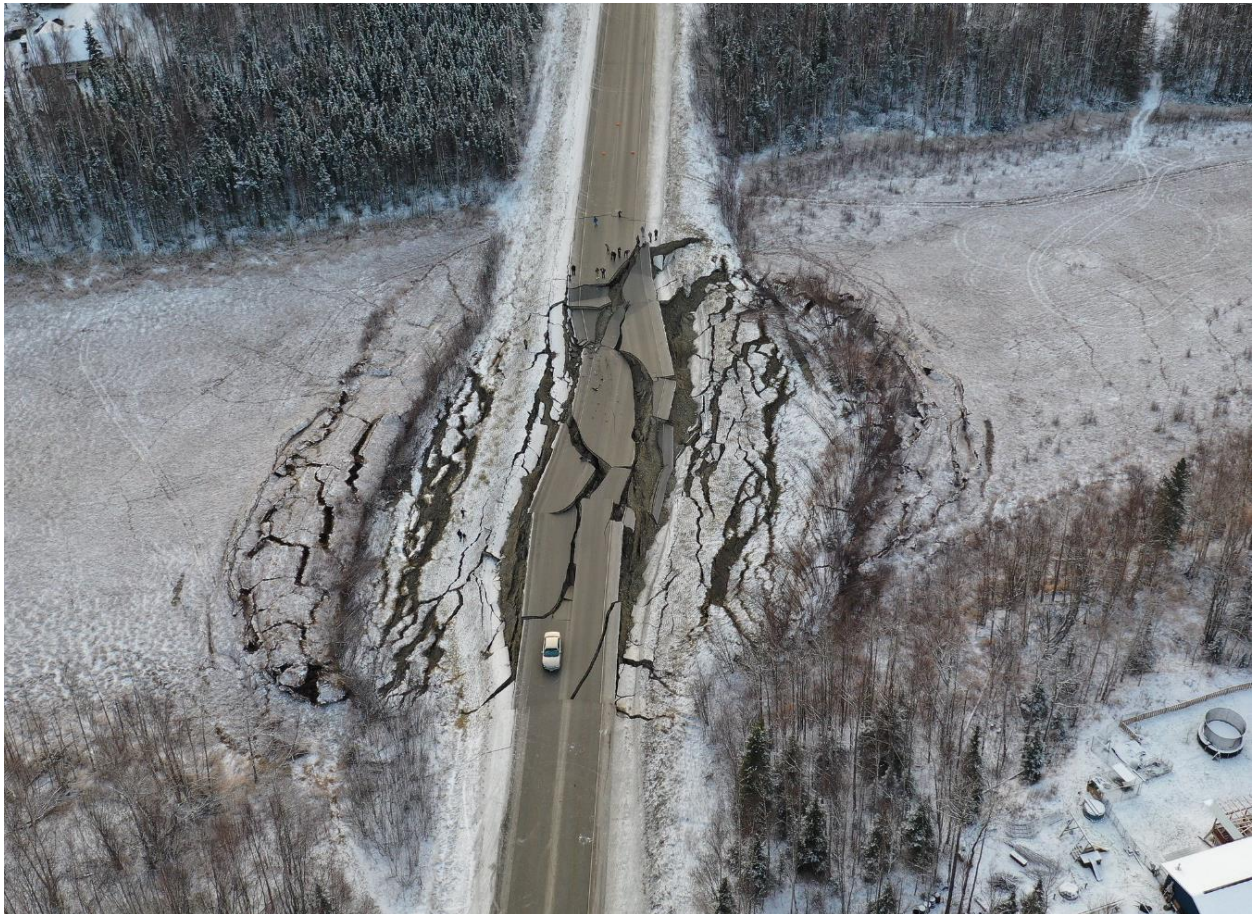
Figure 4.1.4-8: Earthquake Damage on Vine Road Due to Shaking-Induced Soil Failure
